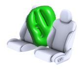
Driver's seat has a far side airbag in addition to the side airbag. Location of far side airbag is shown in the mark.
