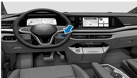
Press the START-STOP button in the center console or remove the ignition key.
