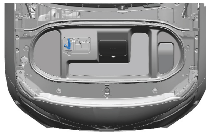
Loosen the screw and pull the battery negative cable.
