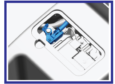
Loosen the screw and pull the battery negative cable.
