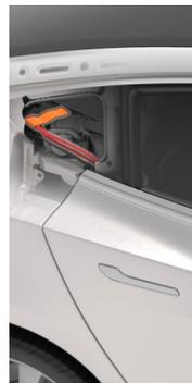
Cut loop is located on the right side of Model Y
