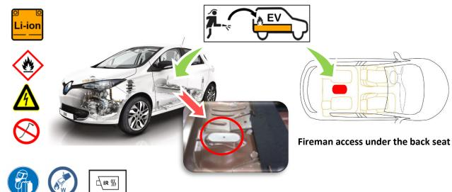
If traction battery on fire : → Water extinguishing by filling
