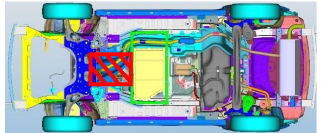
Orange cables area
