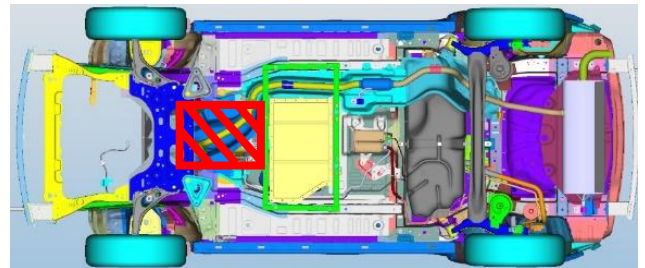
Orange cables area
