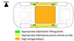
Use caution to ensure you never come into contact with the high voltage battery or other high voltage components while lifting or manipulating the vehicle.
