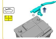
The vehicle power system can be shut down normally.
