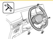
Fully release the locking lever, the steering wheel can be adjusted in 4 directions.
