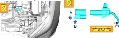
Open the bonnet, pull out the clip from the manual service disconnect(A), press the end of the clip (B) and remove the manual service disconnect.
