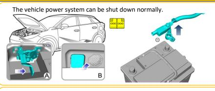
From the inside of the vehicle, pull the bonnet release handle(B), Move the safety catch release handle on the bonnet lock assembly in the direction of the arrow (A) to release the bonnet.
