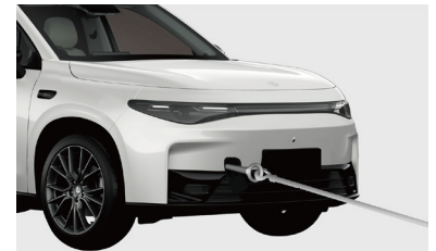
Towing hook installation location
