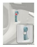
1. Pull the release lever(1) to unlatch the hood. The hood should pop open slightly.
