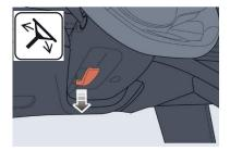
Fully release the locking lever, the steering wheel can be adjusted in 4 directions.
