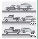
Notice: The use of wheel dollies or flatbed is recommended. Use a wheel lift or flatbed equipment.
