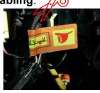
Cut the cable of the service interlock to disable the HV-System
