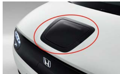
Charge port in the hood
