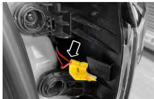
Cut-out connection in the rear of the vehicle behind the right tail light cluster.
