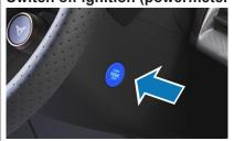
Press the START-ENGINE-STOP button located on the steering column without pressing the brake pedal.
