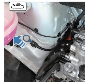
Disconnecting from the charging station (emergency release)
