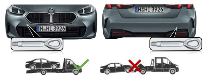
Only use the towing eye supplied in the vehicle and screw in firmly to the limit position.
