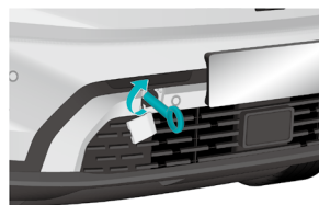
Tow hook installation location
