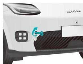
Hook installation position
